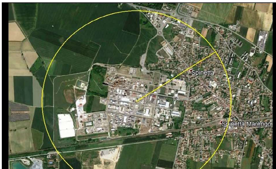
ZONA DI DANNO IDLH (IMMEDIATELY DANGEROUS TO LIFE AND HEALTH)
